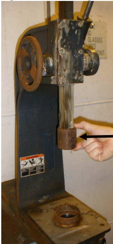
Fig. 5: Metal disc for pushing on core material.
