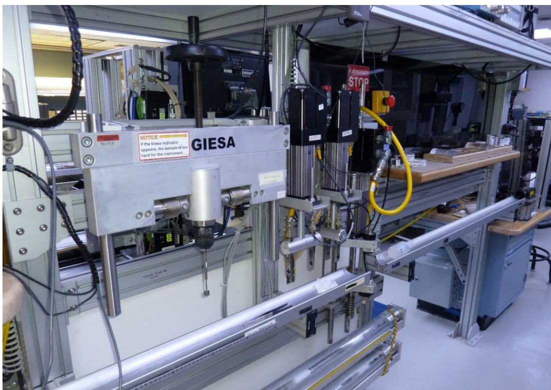
Figure 48. Sonic velocity and Shear strength instrumentation (Gantry)
