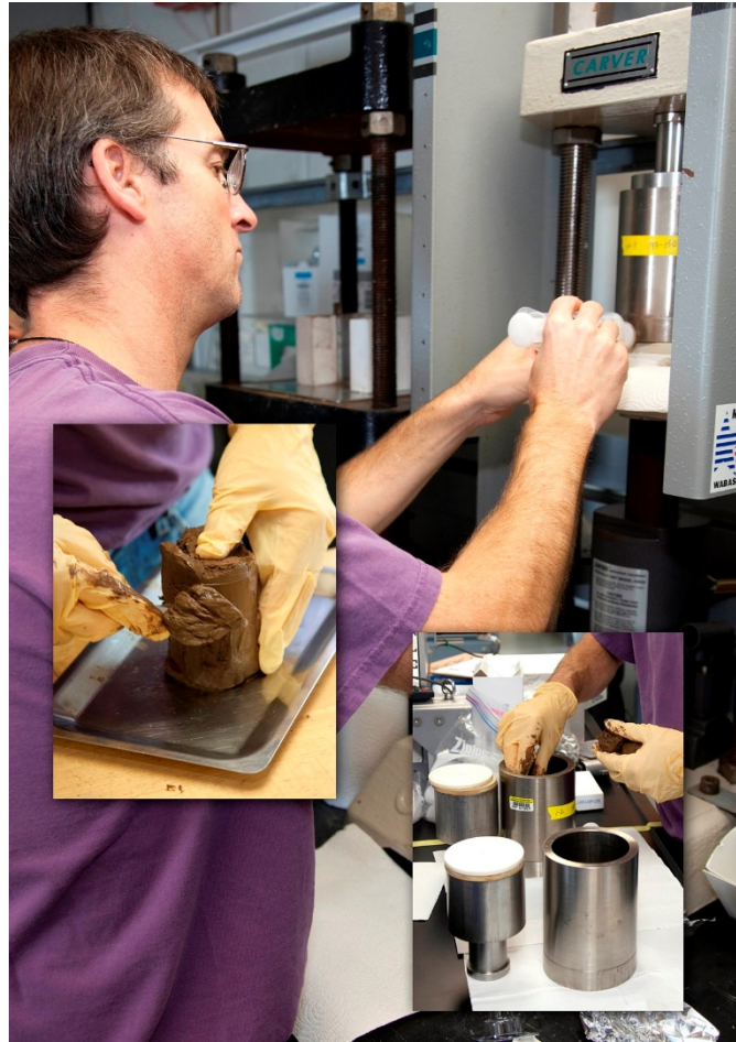
Figure 36. Process of scraping from side, putting the pressure vessel and attaching the syringes for posterior squeezing of samples to take the interstitial water from them.
