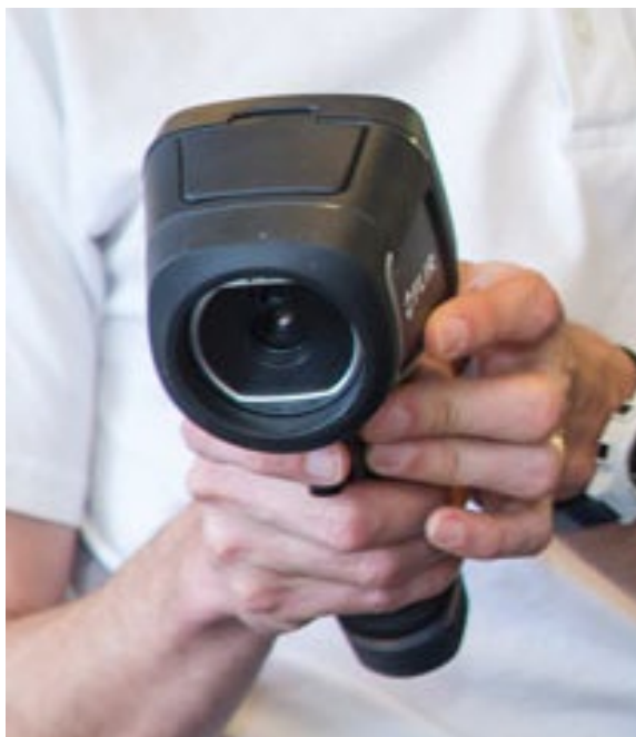
Figure 39. Infrared Camera for detecting clathrates
