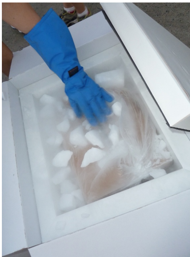
Figure 7. Example of a World Courier box with a styrofoam insert filled with bagged samples in a plastic bag to protect from dry ice.
