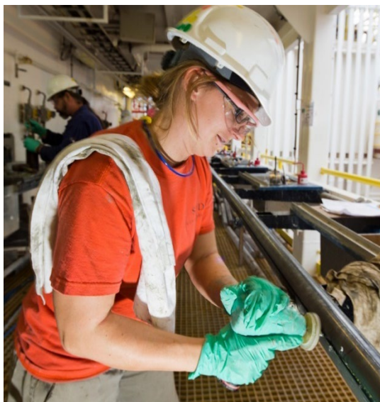
Figure 24. Drilling holes in liner
