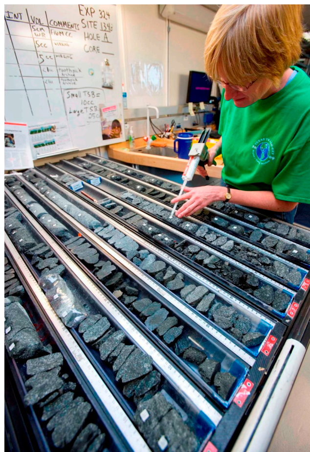
Figure 61. Gluing hard rock labels
