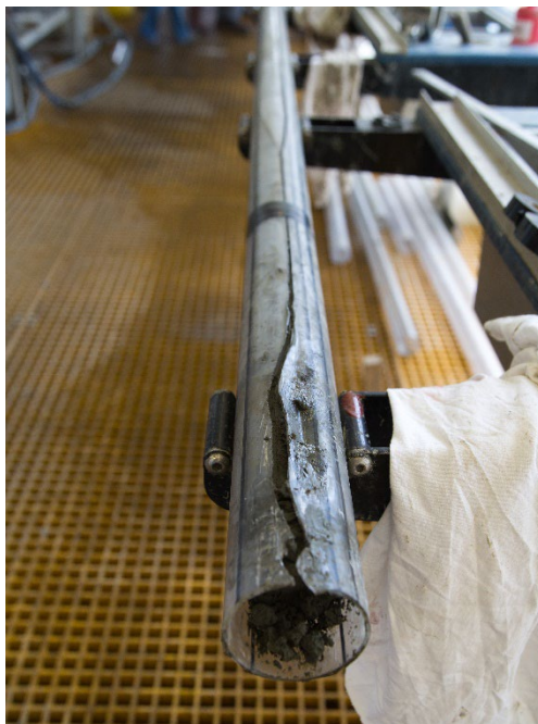
Figure 26. Example of a shattered liner
