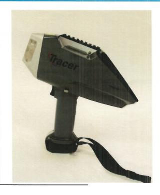
General instrument performance may be checked by taking a measurement of the supplied silver sample. The measured value for each element should be within the acceptance limits shown above. If not, contact Bruker for support. Email: service.hmp@bruker.com.
