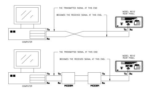
Figure 4-2 Serial Port Connection Schemes
