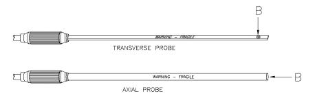
Figure 1-3 Hall Probe Configurations
