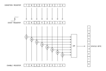
Figure 4-3 Condition, Event and Enable registers
