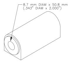
Figure 2-1 Zero Flux Chamber
