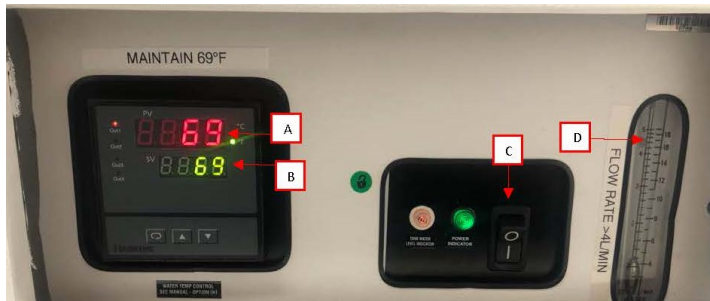
Figure 4. HASKRIS Control Panel. (A) Actual temperature. (B) Set temperature. (C) On/Off switch. (D) Flow meter
