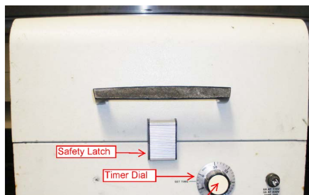
Figure 9: 8000M mixer mill. (A) Safety latch (B) Minute timer (C) Seconds timer (D) Start button (E) Pause/Stop button (F) Timer countdown LCD display.
