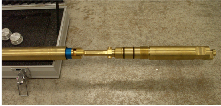
Figure 9B: slide the key end of the other end seal onto the Flexit tool, insert it into the barrel and tighten. Hand the assembly to the Core Tech for final rigging with the snubber shock and IODP pressure case.
