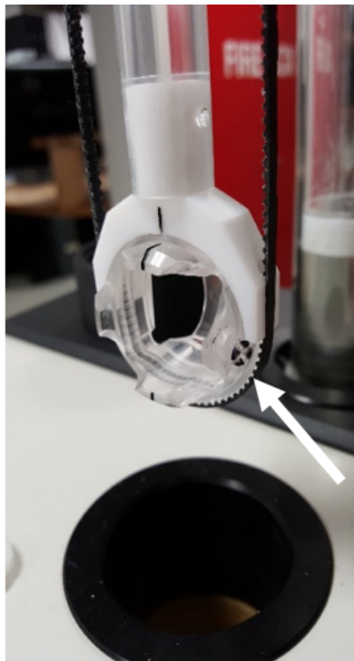
Figure 7 Empty Kappabridge Holder prepared for holder measurement.
