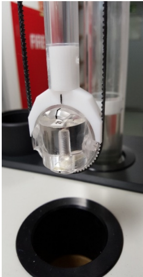
Figure 5 Kappabridge Holder with calibration standard.
