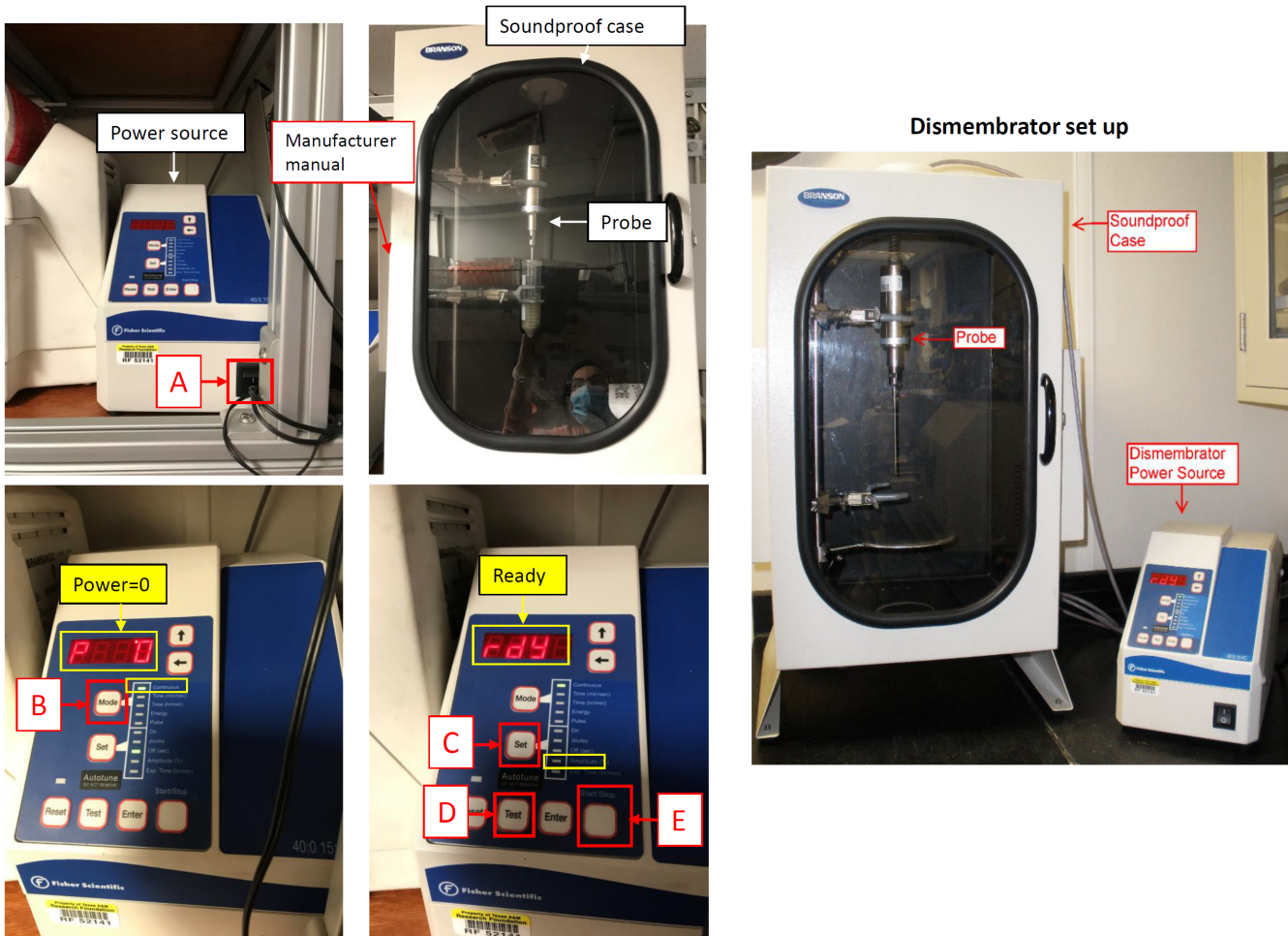
Figure 10. Dismembrator set up and Probe with power source. Dismembrator power source control Panel. (A) On/Off switch (B) Start button (C) Set button (D) Mode button (E) Start/Stop button
