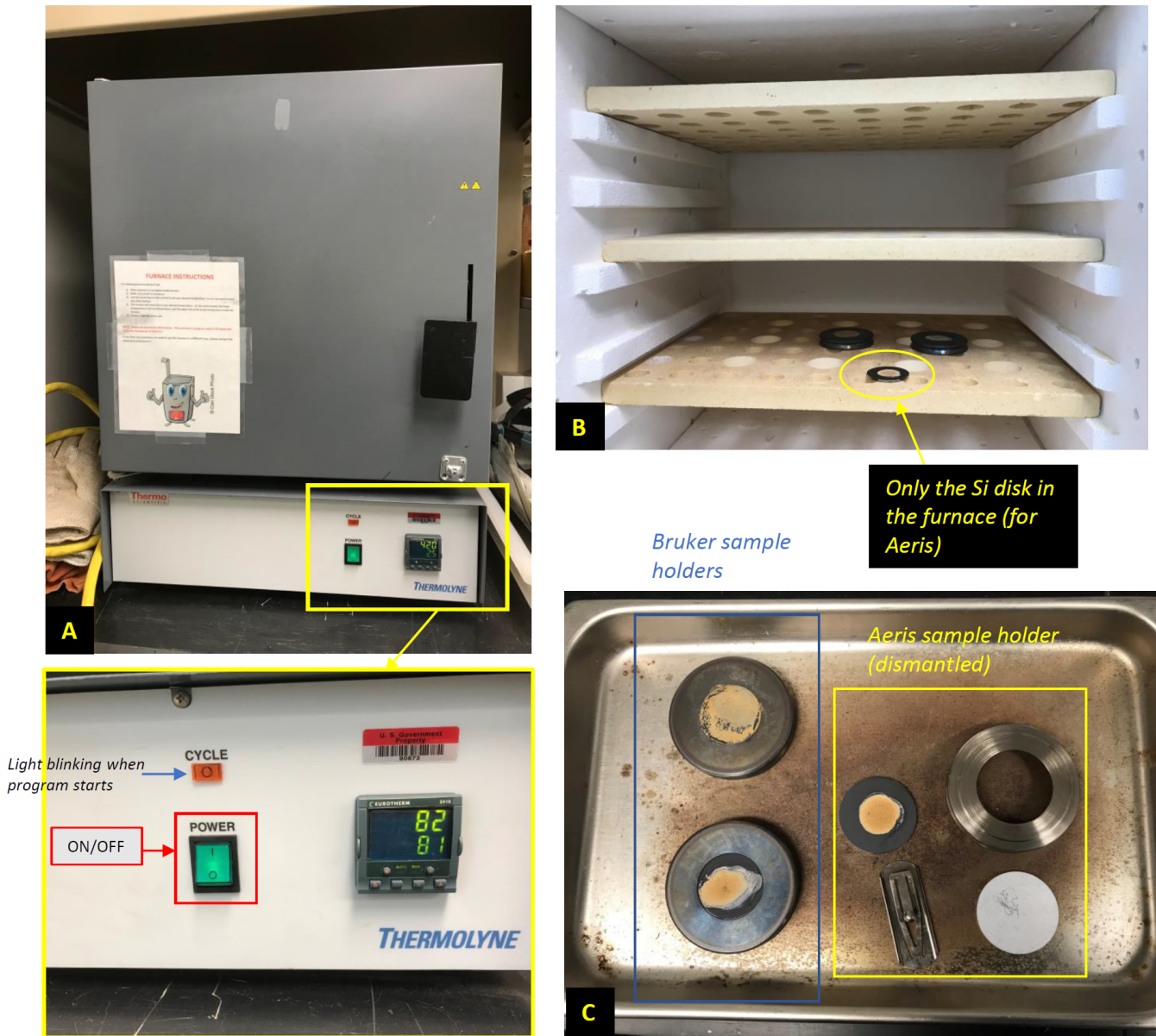
Figure 16. A. Muffle furnace in the Chemistry Lab. B. Clay Mount in the muffle furnace. Note that only the Si disk of Aeris sample holder is put in the furnace. C. After heating.
