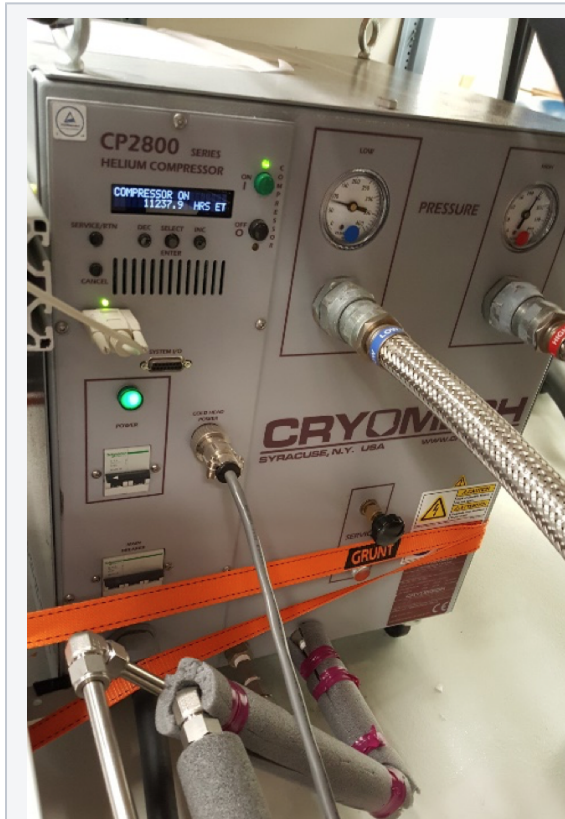
Figure 1a: Cryomech 2800 Series Compressor for SRM. The compressor is located at the aft end of the paleomagnetism lab just behind the load end of the SRM track.
