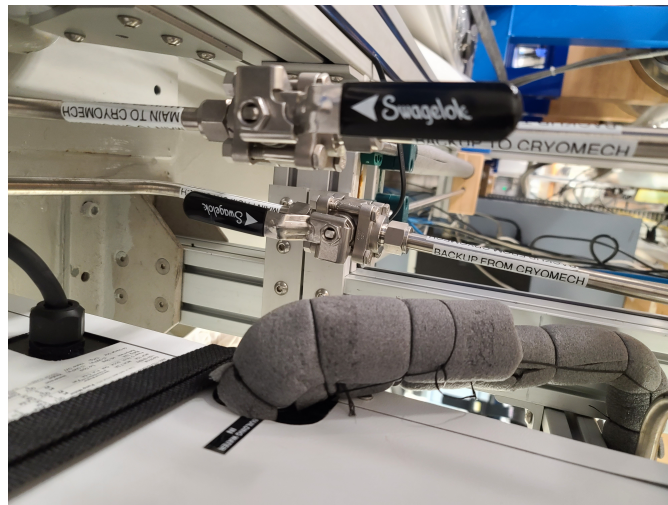
Figure 10: The "from cryomech" line switched to the backup system by turning its black selector valve down 180°.
