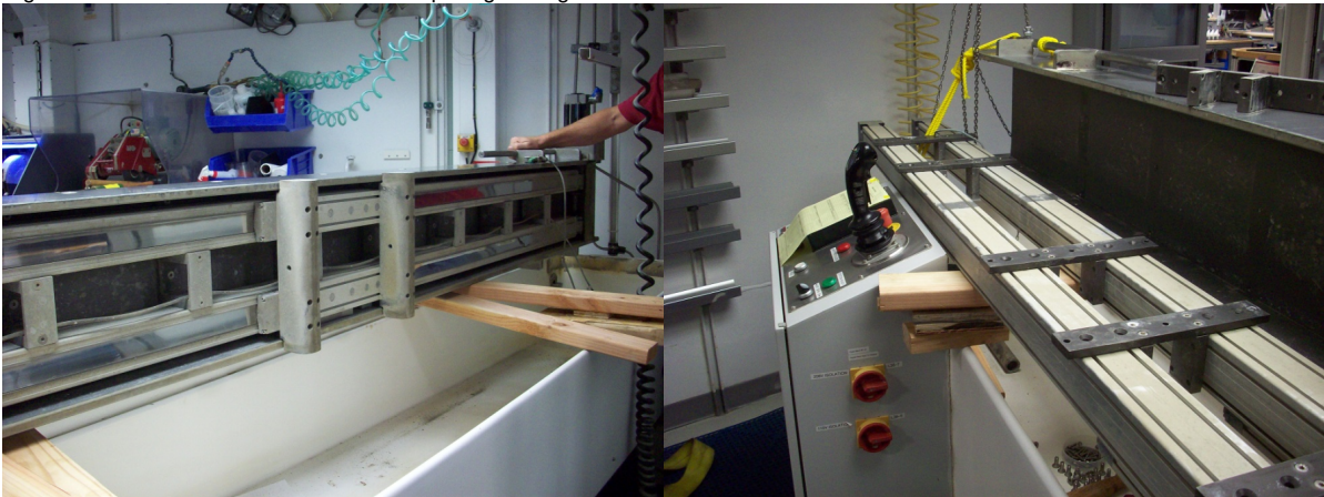
Left: Underside of the splitter showing linear actuators and travelling blocks for the splitting carriage. Right: Top of the linear actuators with the brackets that attach them to the splitter frame.
