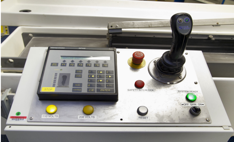
Figure 2. Joystick and RP240 Operator Interface mounted on Control Unit.
