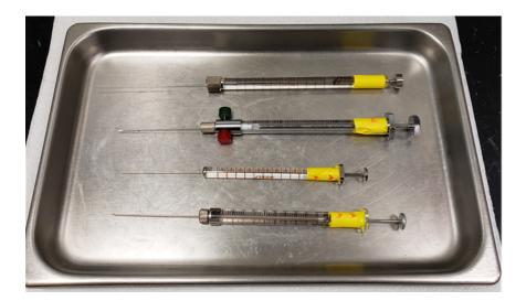
Figure 5: Different syringe types for preparing PFT standards and for injecting samples. Listed from top to bottom: 1 μL glass analytical syringe from Scientific Glass Engineering (SGE), 0.5 mL Teflon-fitted Pressure-Lok glass syringe from Precision Sampling Corp, 10 μL glass analytical syringe from SGE, 0.10 mL (100 μL) Microliter #710 glass syringe from Hamilton Co.
