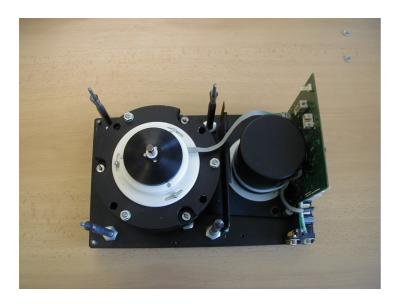
Remove the upper rectangular plate with coil and sample manipulator.
