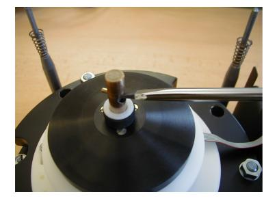
Remove the screw used for fixing the holder to the shaft of the rotating system (carrier pin), remove also the white teflon and black rubber washers.
