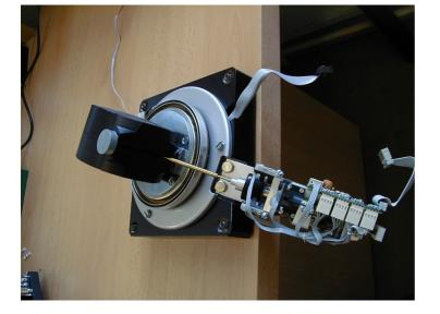
Put the rectangular plate with coil and sample manipulator on the corner of the desk to prevent any demage.
