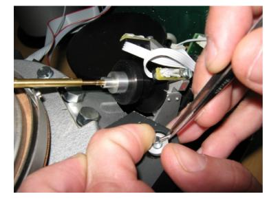
Push the upper plate in each particular corner and remove the security pin. Put the spring, small metallic plate and security pin on the desk in square pattern corresponding the position of these parts on the device. Please be careful to remember position of springs to be able to place them to the same positions reassembling the device.
