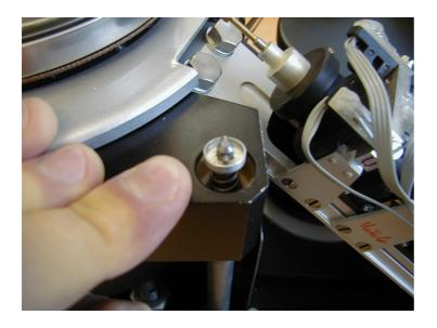
Release four springs in the corners of the rectangular plate.
