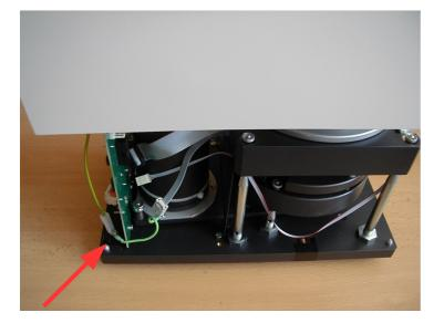
Do not forget to unplug the yellow-green ground cable (marked by the red arrow).
