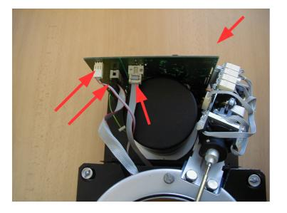
Unplug all the cables connected to the electronic board (marked by the arrows).
