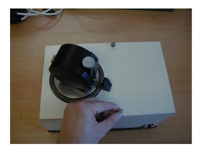
Switch the device off, unplug the mains cord from the power supply. Open the pick-up unit by unscrewing the safety screws and removing the cover.
