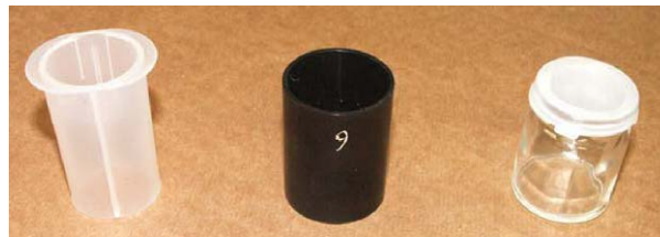
Figure 6. Sampling tool (left), aluminum cup, and Wheaton vial for MAD measurements.
