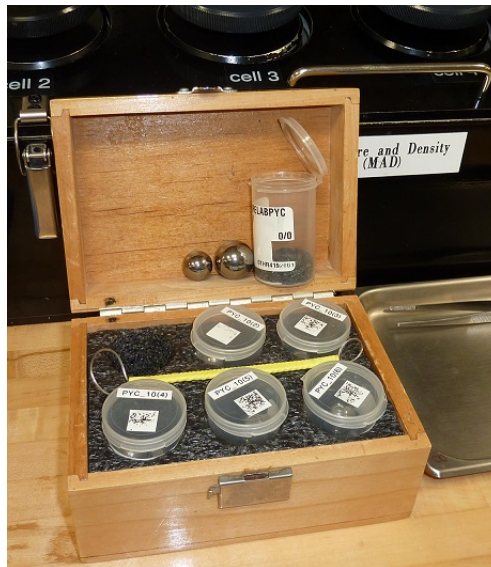
Figure 23. This box contains six sets of steel balls and the wire tool to extract them from the cells.
