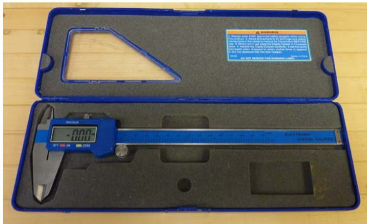
Figure 3. Precision Digital Caliper for Measuring Dimensions of Certain Samples.
