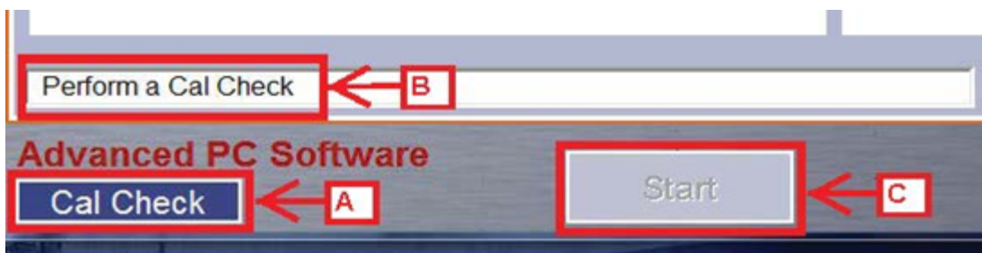
Figure 8. Cal Check Indications. A. Cal Check Measurement Button. B. Message to perform Cal Check. C. Disabled Start Button
