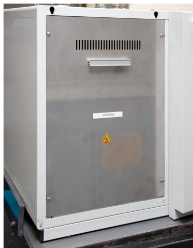
Figure 4. Furnace Compartment Access with Protection Plate WARNING! Do not open the furnace compartment during operation
