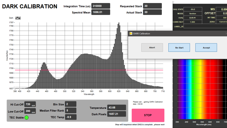
Figure 4. QE Pro Dark Calibration.
