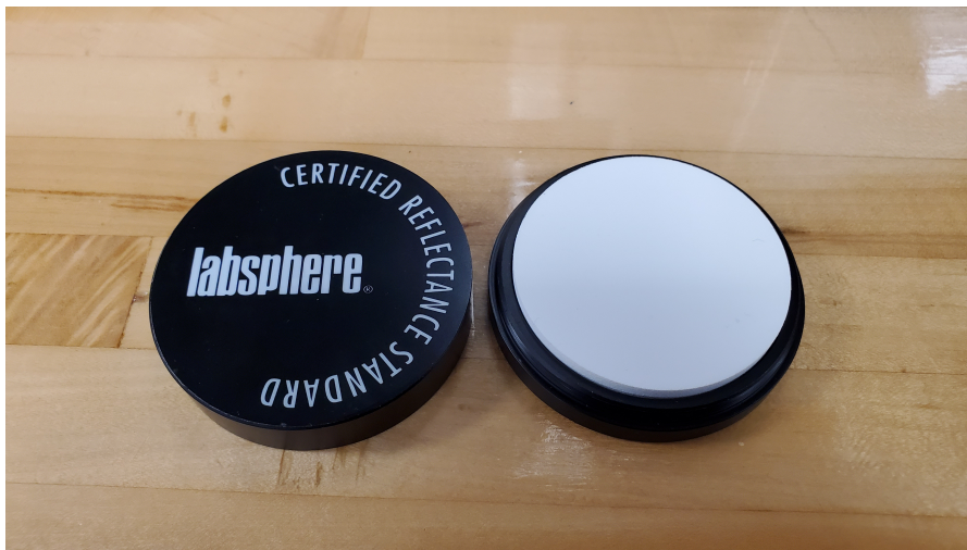
Figure 2. WHITE Spectralon® Calibration Standard
