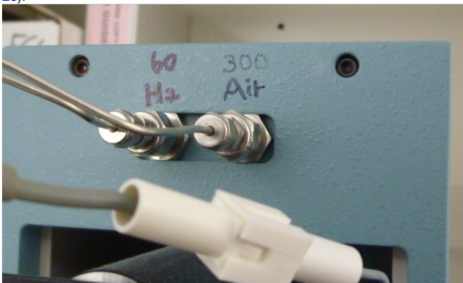
Figure 24. Gas Terminals Connected to the Front.
