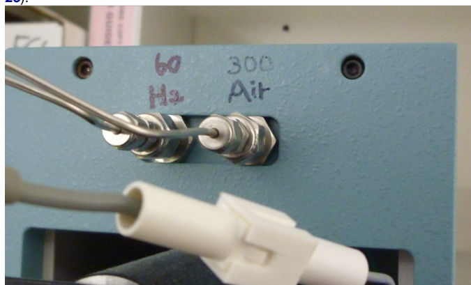
Figure 24. Gas Terminals Connected to the Front.
