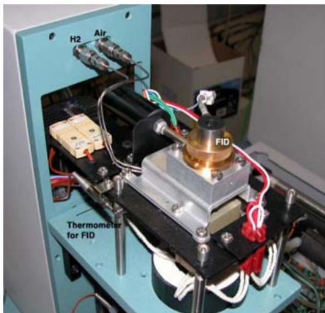
Figure 10. Internal View from Top of FID Unit.
