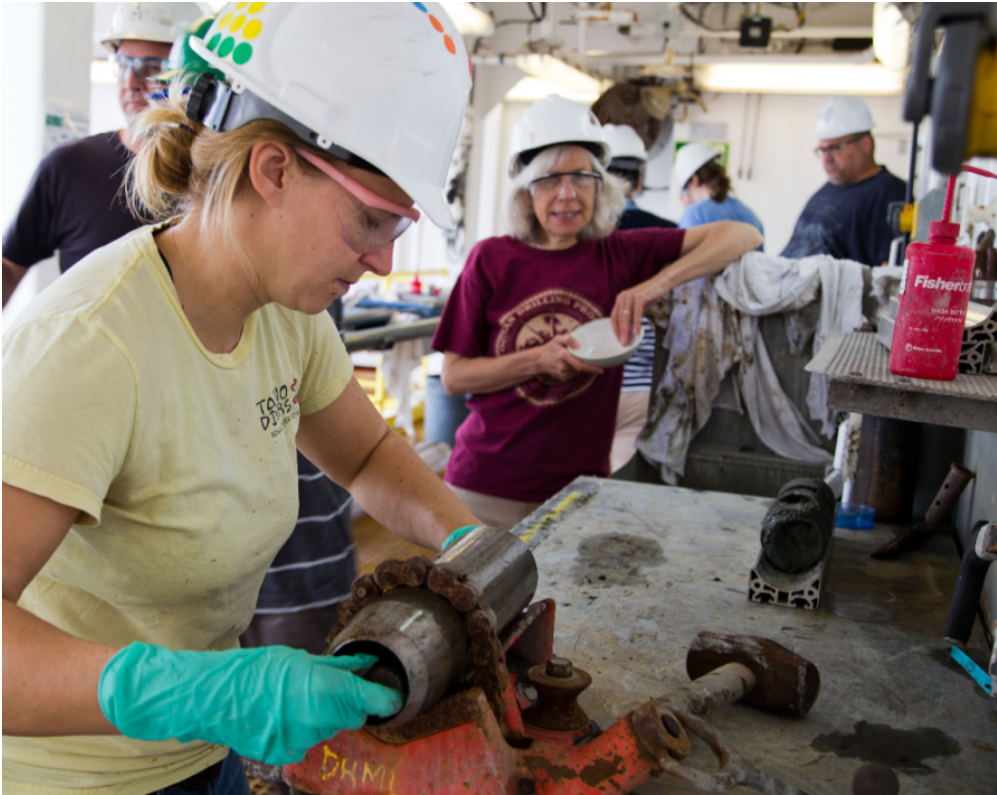
Figure 1: Extruding core catcher material at the core catcher bench; notice the Paleontologist waiting with white bowl – give PAL sample to paleontologist.
