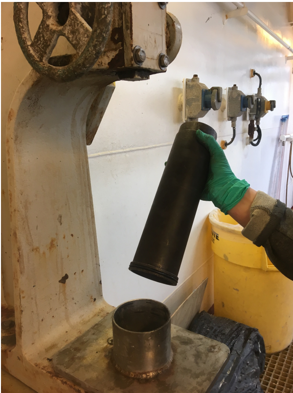
If the press is unavailable the old XCB sleeve tool needs to be used to get the inner rings out of the sleeve. Note that the sleeve must be turned around on the chain vice to get the lip of the flange to catch the vice and be stable. Wet the tool.
