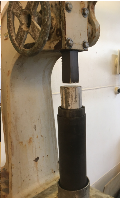
If the press is unavailable the old XCB sleeve tool needs to be used to get the inner rings out of the sleeve. Note that the sleeve must be turned around on the chain vice to get the lip of the flange to catch the vice and be stable. Wet the tool.
