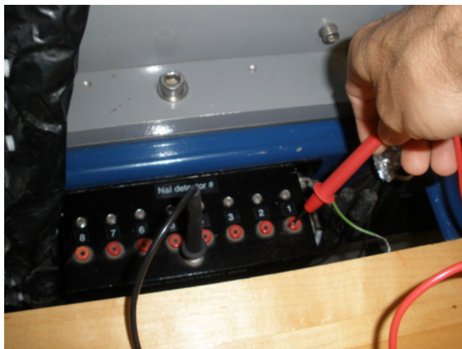
Figure 32. Insert the multimeter probes into the bias detector box to measure the voltage. Black to white. Red to red
