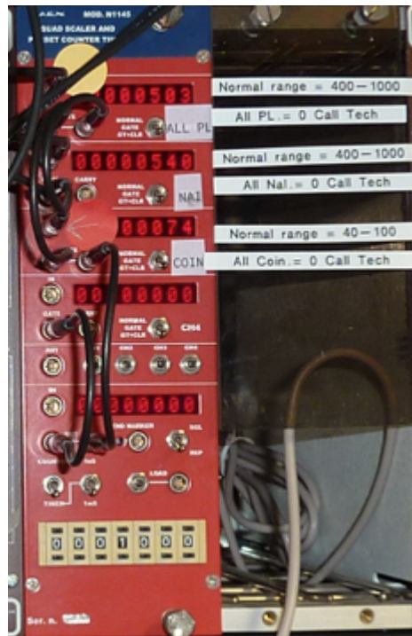
Figure 8. CAEN signal counter depicting summed plastic, NaI, and coincidence values
