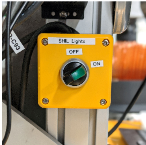
Figure 35: Hardware Switch to turn power on or off to the lights located behind monitor.
