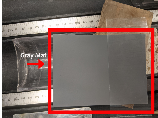
Figure 47: The Gray silicone mat being cleaned with tape.
