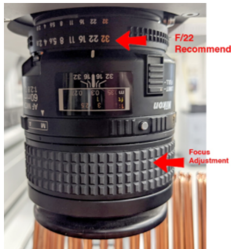
Figure 22: Setting the F Stop on the Camera. Note that F/22 was recommended by the camera manufacturer but that value is debated. F/16 is the preferred value by the imaging specialists onboard. Darker cores may need F/22.
