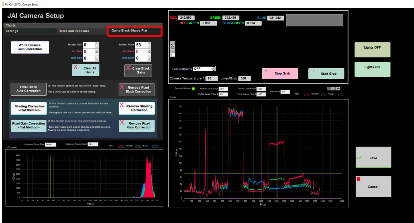
Figure 36: JAI Camera Setup Window showing the Gains-Black-Shade-Flat tab. The Gains-Black-Shade-Flat tab is outlined in red.
