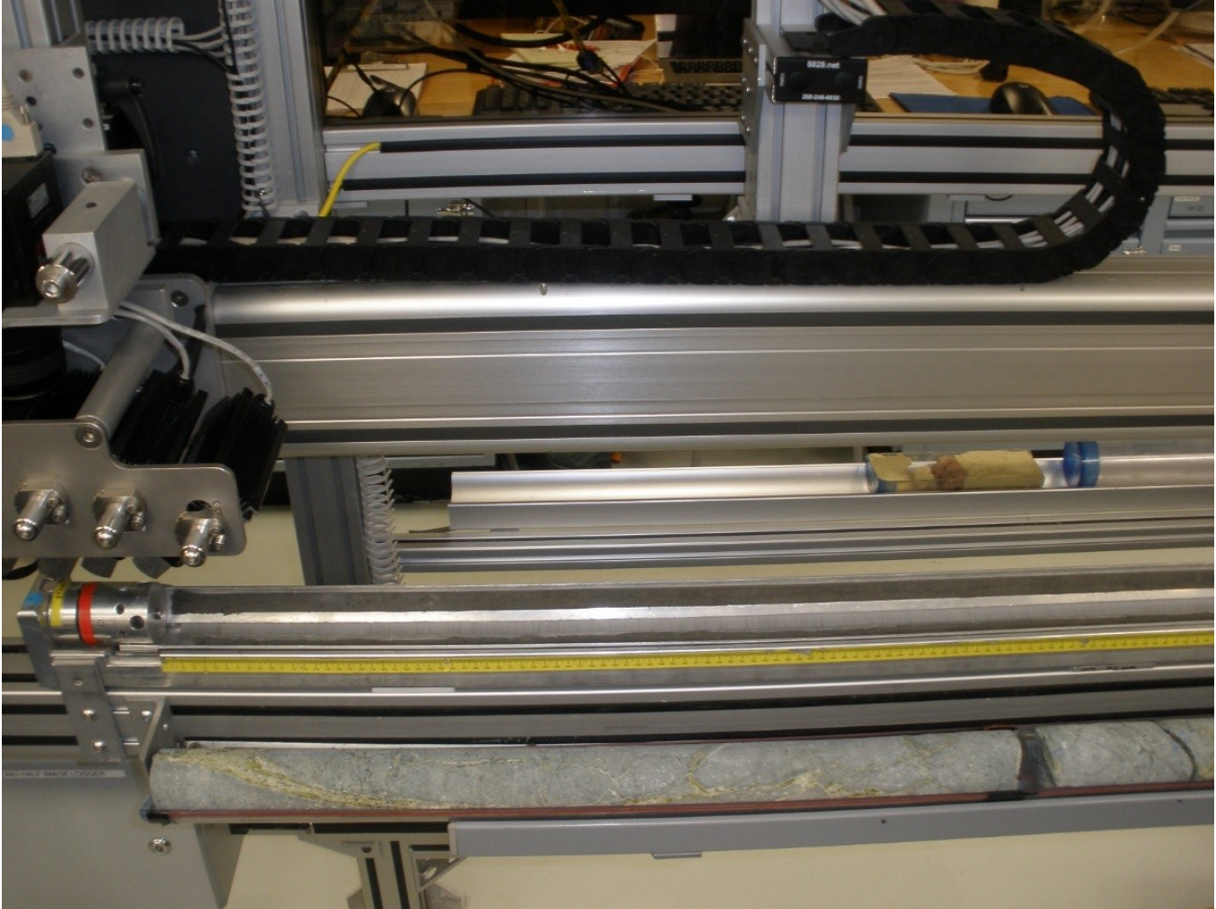
Figure 16. Whole round core correctly placed on the split liner section.
