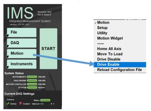
Figure 27. IMS commands to enable motor
