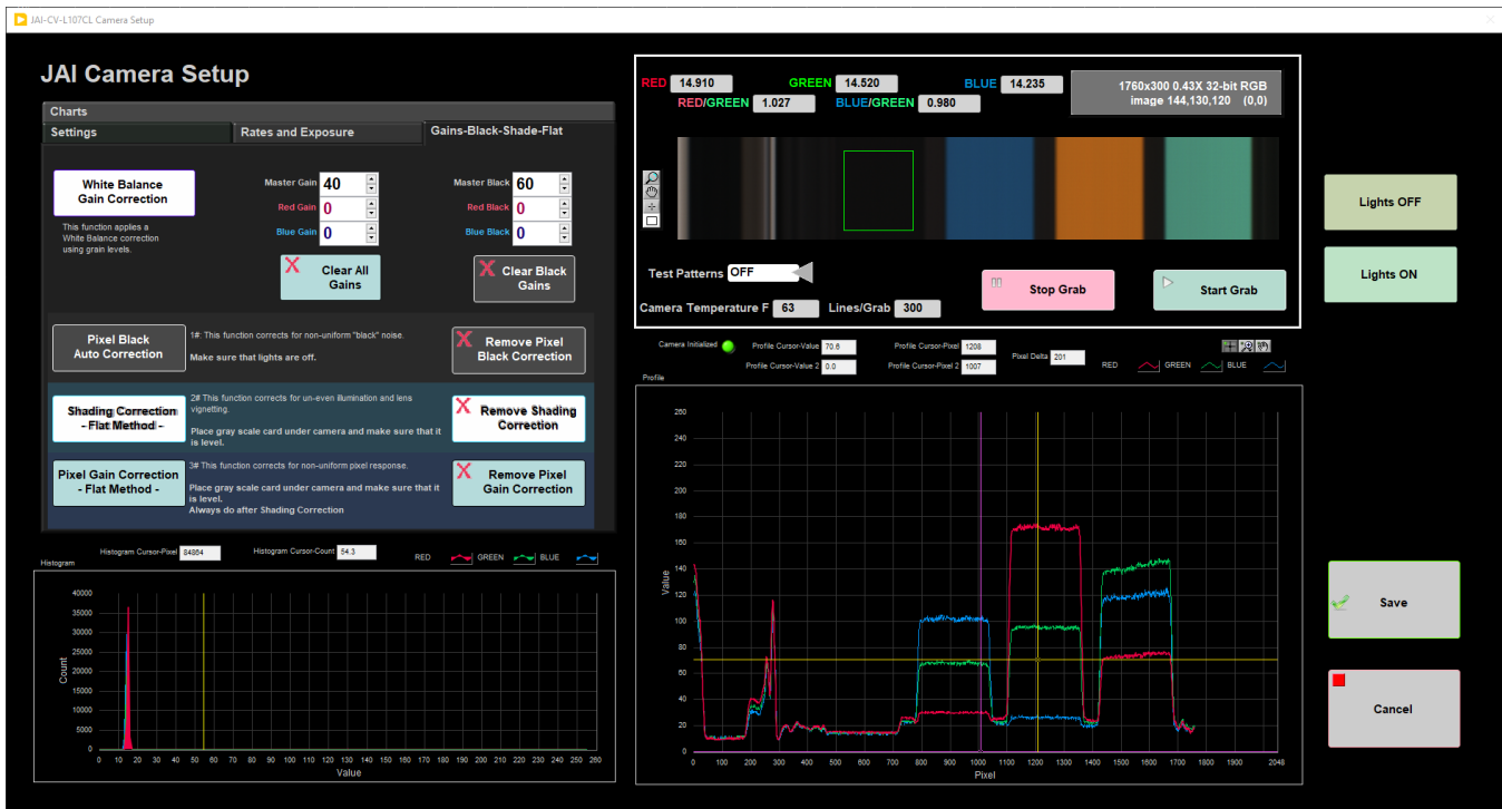
Figure 23. Adjusting Master Black, RedBlack and BlueBlack to reach RGB values of 15 for black square.
