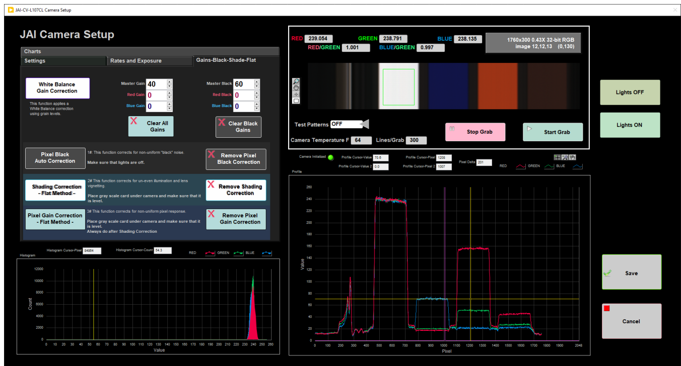
Figure 22. Adjusting Master Gain to bring the Blue values up to 240.
