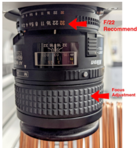
Figure 16. Setting the F Stop on the Camera. Although the figure says f/22 is recommended (recommended by the manufacturer) onboard we found f/16 works best for our scanning needs.
