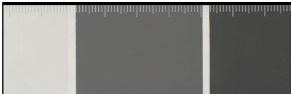
Figure 10. QP 101 card showing centimeter marks for pixel pitch calibration.
