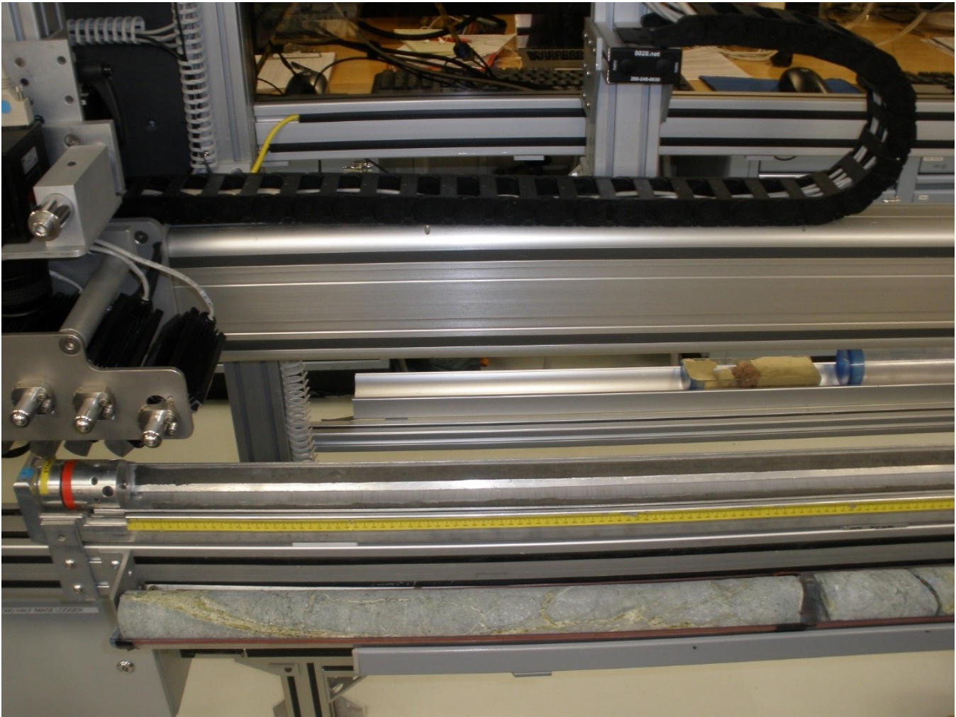
Figure 45. Whole round core correctly placed on the split liner section.
