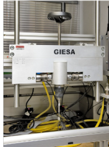
The Giesea FL2 Frame and blade component of the Automated Vane Shear (AVS) equipment.
