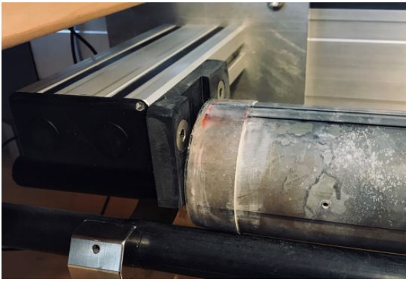
Figure 3. Blue end cap near the top-of-section sensor, clear end (bottom of section) touching the pusher.
