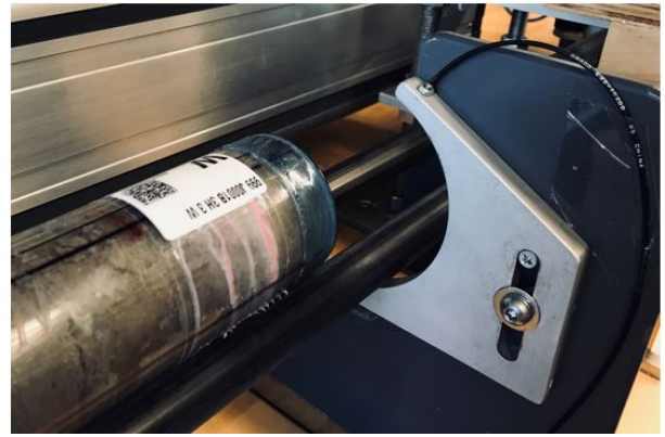
Figure 3. Blue end cap near the top-of-section sensor, clear end (bottom of section) touching the pusher.
