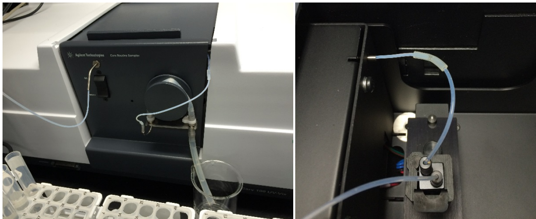
The SP3 is connected to Cary unit via RSA sample inlet tube.
