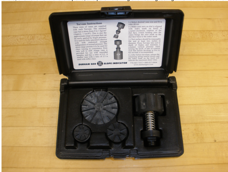
Figure 13. Torvane Shear Device.
