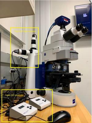
LEDs are switched on and off by pressing the 'on/off' button located on the left side of the microscope. At start-up the pE100 light source will revert to the same settings that were set when it was last powered down. New light sources are supplied with the settings as shown below.
