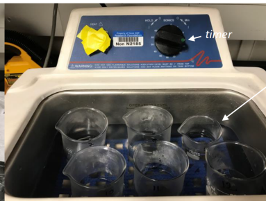
3. Sonicate the samples with isopropyl alcohol inside or DI water for 15-20 minutes
