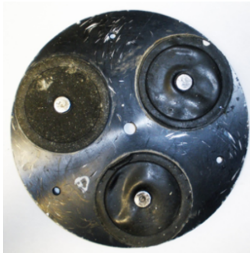
Figure 9. Three-pinned rack plate to hold three small vessels in the Shatterbox
