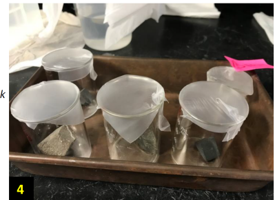
4. Cover the beakers with Parafilm after drying oven at 110°C for about 12 hours
