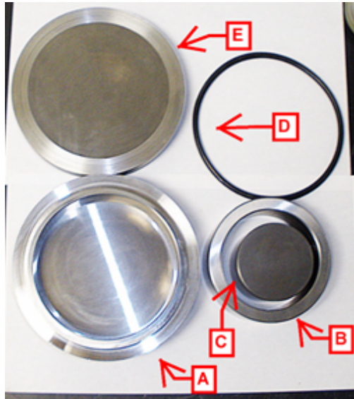
Figure 8. Large Vessel components. A. Container B. Inner Ring C. Puck D. O-Ring E. Lid
