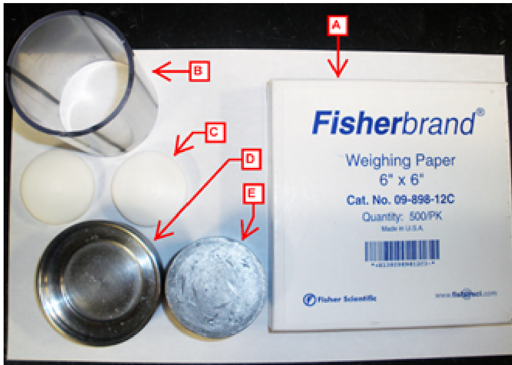
Figure 2. Materials needed for assembly of 'crushing unit'. A. Weigh Paper 6"x6". B. Core Liner C. Two Delrin Discs D. Stainless Steel Base E. Aluminum Die
