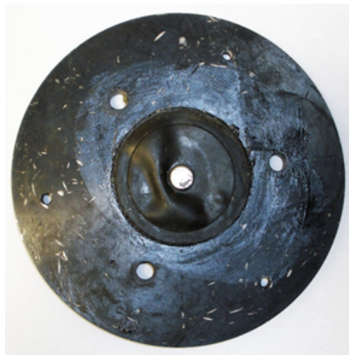
Figure 9. Three-pinned rack plate to hold three small vessels in the Shatterbox
