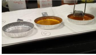
Stage 1: 1.5% HCI: Using large tweezers, dip the entire face/side of the billet or slide that is to be stained. For the other stages it is important to only dip half way but for this stage, since it doesn't stain, it can be done on the entire surface. Hold in the HCI for 10-15 seconds and then rinse with DI or nannopure water. I found it best to place a large beaker under the handheld nanopure dispenser and rinse the slide or billet off in the water stream, and not dunk it into the beaker.
