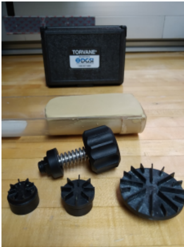
Figure 2. Vane driver and the 3 kinds of vanes.
