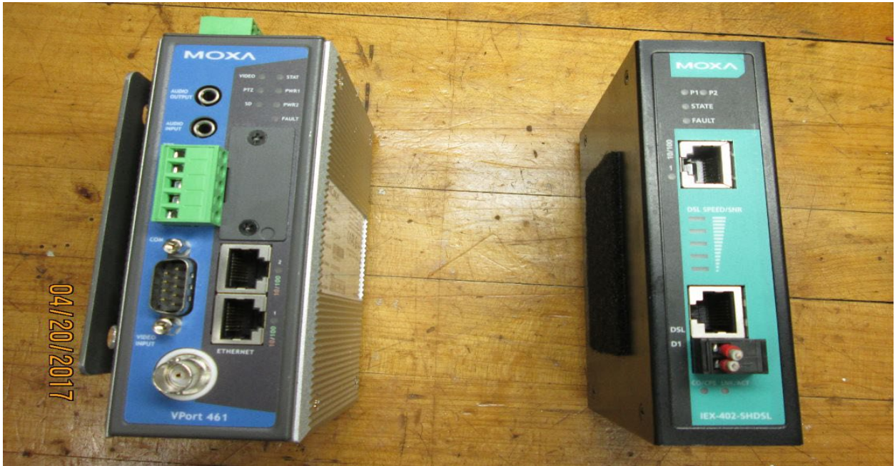
Figure 7. Photo of the Moxa Video Server (Left) and ADSL Modem (Right).
