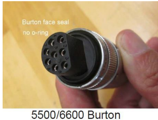
Figure 16. 5500/6600 Burton Connector (No O-Ring).
