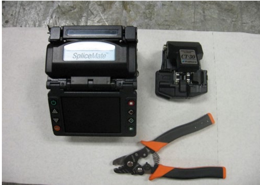
Figure 24. Fusion Splicing Tools.
