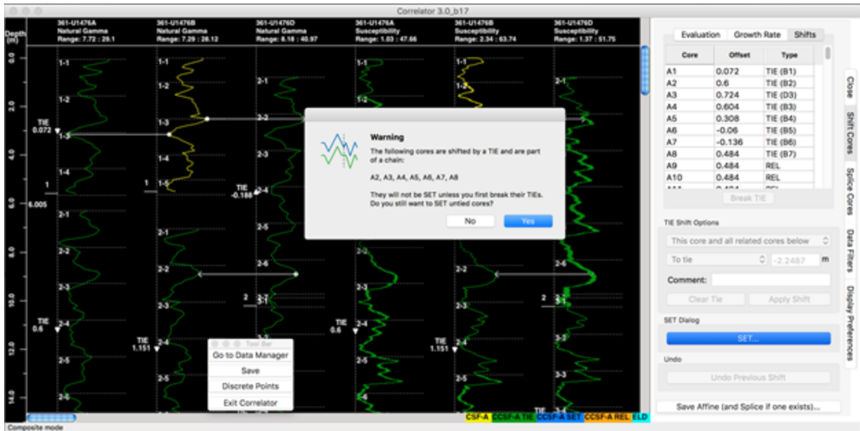
Figure 3-33. The attempt to SET cores that are part of a chain failed.
