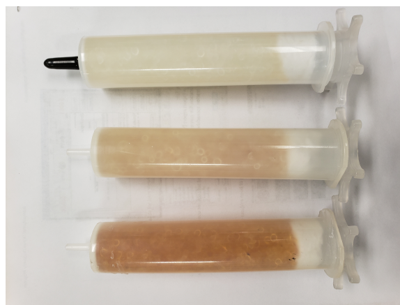
Figure X: Example of H 2 O scrubbers used in-line with the MSM air inlet. From left to right: a regenerated scrubber ready to use, a scrubber removed from the instrument which must be regenerated, a new scrubber which must be regenerated before use.
