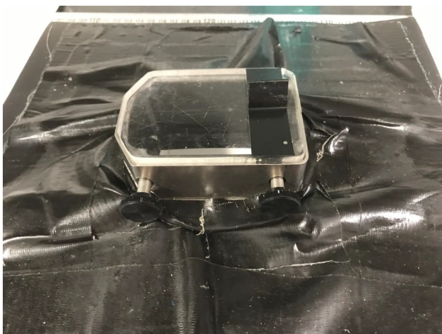
Figure 13. Measuring the offset. A. Lead mat with offset window. B. Offset window (crossing point of the blue lines is the offset)
