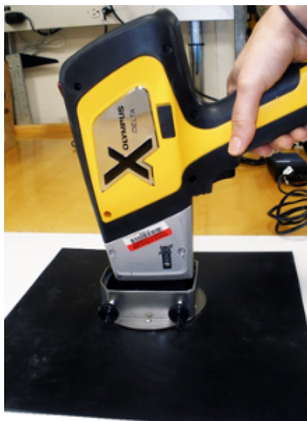
Figure 14. pXRF being lowered into section half shielding. pXRF oriented with indents facing set screws.
