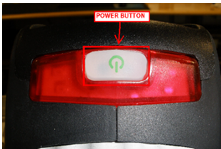
Figure 5. pXRF power button outlined in red. pXRF is off in this figure.
