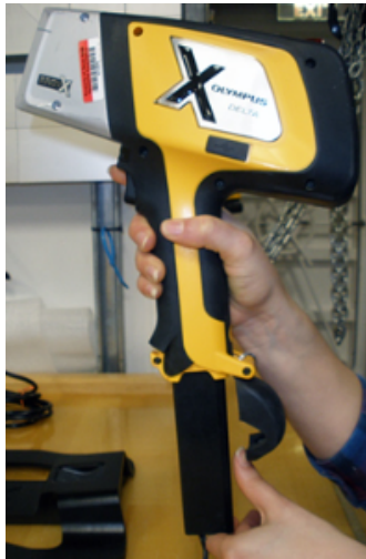
Figure 4. AC battery source inserted into pXRF
