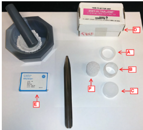
Figure 14. Mortar and pestle along with scoopula. XRF Sample Cup components denoted with red arrows A. Open-end Ring B. Cup C. Cap D. Ultralene® film box E. Whatman Filter Paper F. Foam plug inserts
