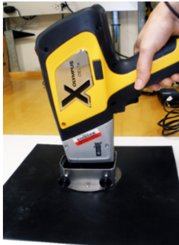
Figure 13. pXRF being lowered into section half shielding. pXRF oriented with indents facing set screws.
