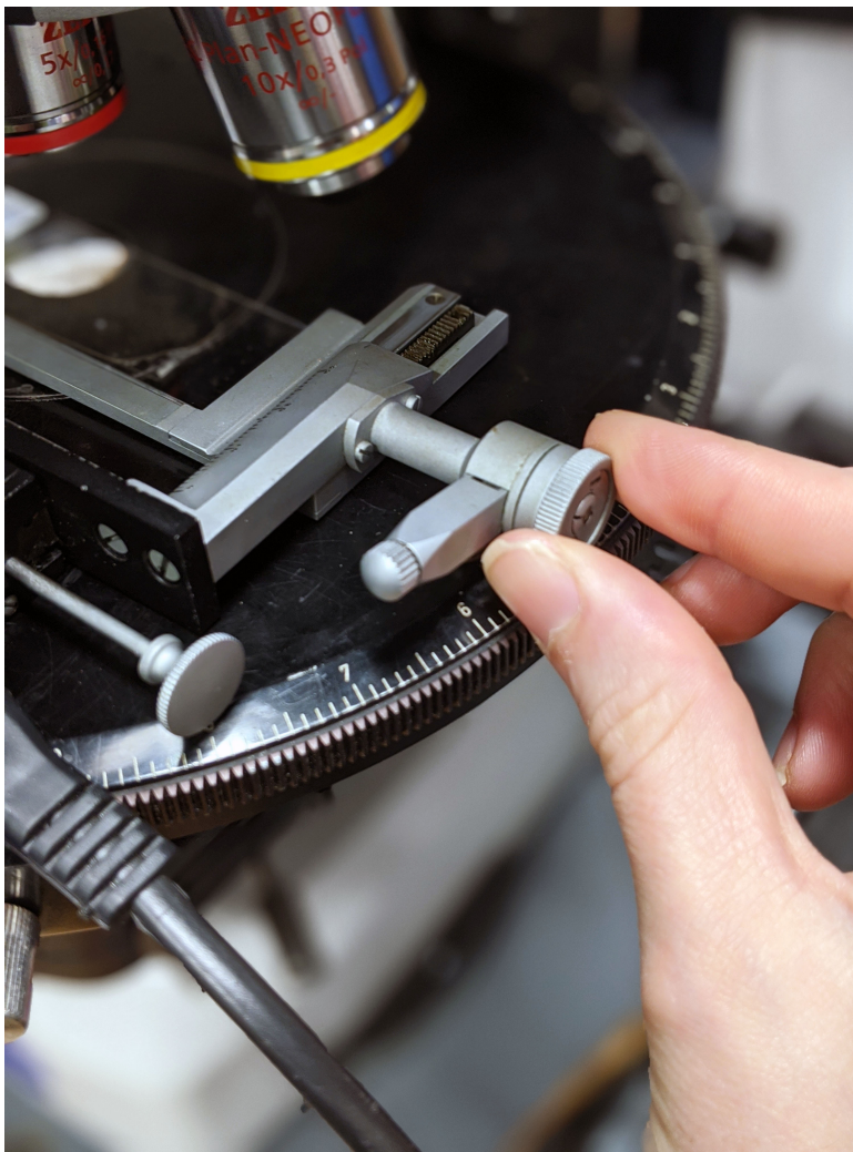
Figure 16: Wheel being turned to move sample up.
