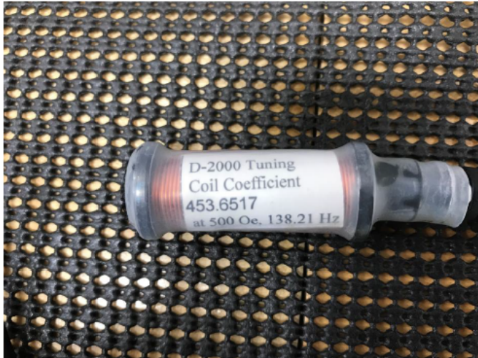
Figure 9. Tuning coil in the sample holder to be at a good location for tuning
