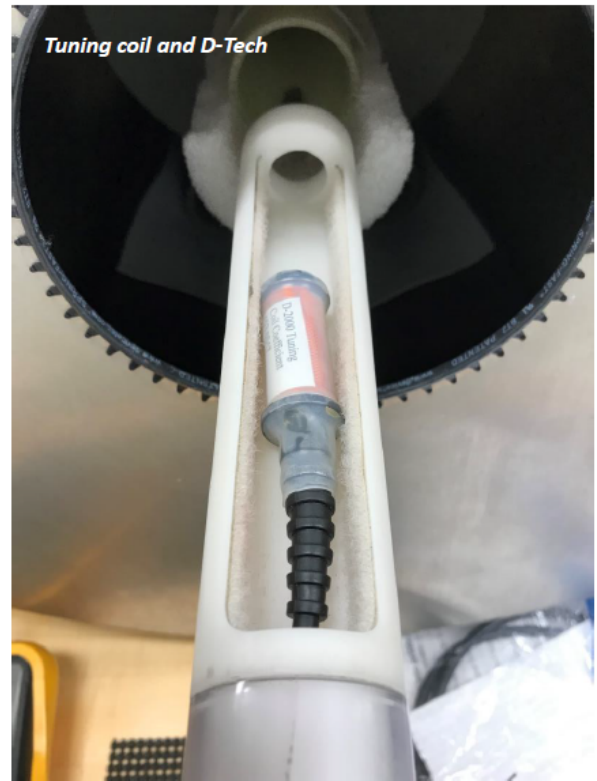
Figure 9. Tuning coil in the sample holder to be at a good location for tuning
