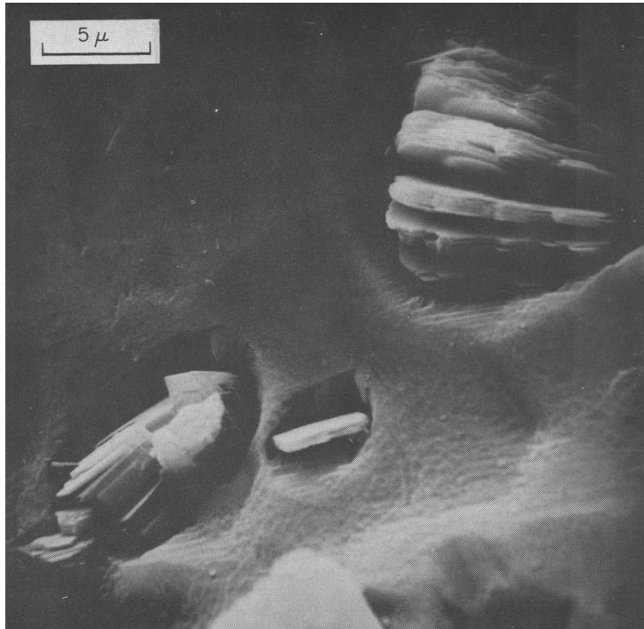
Fig. 5(a). Normal view of pyrite cleat surface with kaolinite packets growing through; Herrin (No. 6) Coal Member, Carbondale Formation, Sangamon Co., Illinois (Pennsylvanian).
