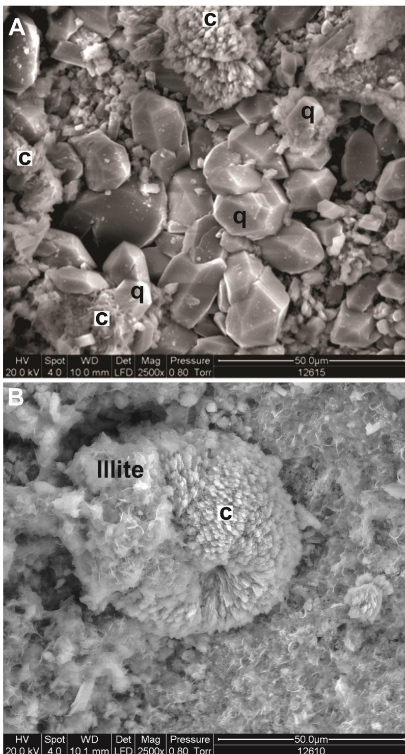
Figure 1: SEM images of core from a geothermal field. (A) The formation of quartz (q), bladed calcite (c), followed by further quartz formation. (B) Illite visible on top of bladed calcite (c) indicating it formed after the calcite.
