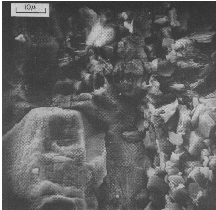
Fig. 4(a). Cross section of cleat containing kaolinite (right) and pyrite (left) from the Herrin (No. 6) Coal Member, Carbondale Formation, Sangamon Co., Illinois (Pennsylvanian).
