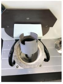
2. Remove the cover attached to the furnace body. (There are fixing screws on both sides)
