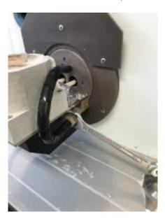
5. Remove the motor box from the furnace body by loosening the three screws.
