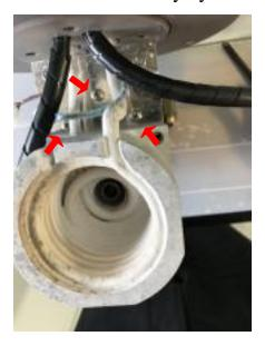
6. Remove the front cover and expose the rotating part
