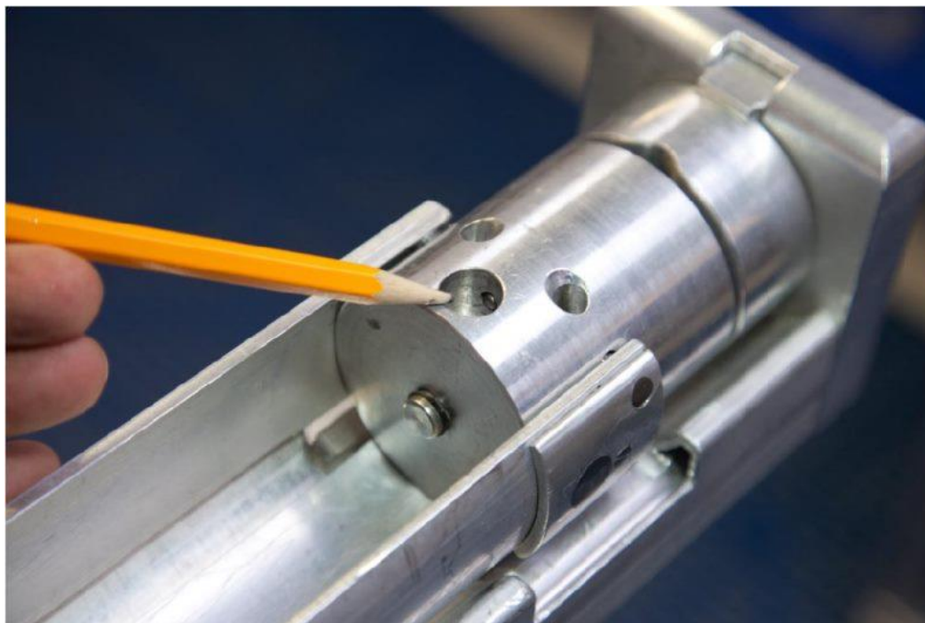
Figure 55. Aluminum frame used for holding whole-round core pieces for imaging, Expedition 345. View of one end of the frame, with one of the four bracing strips removed, as would be the case while imaging the outer core surface.
