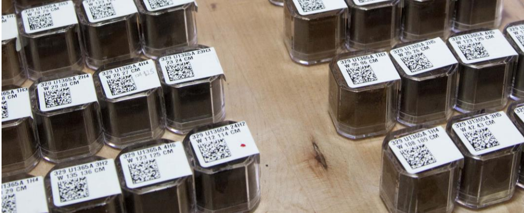
Figure 50. Example of paleomagnetic cubes. Samples taken in soft sediment.
