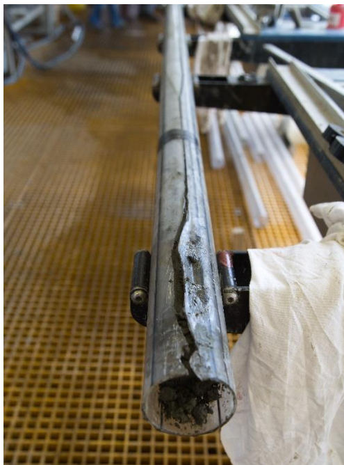
Figure 26. Example of a shattered liner
