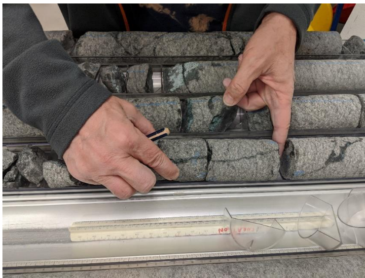
Figure 56. Piecing together hard rock
