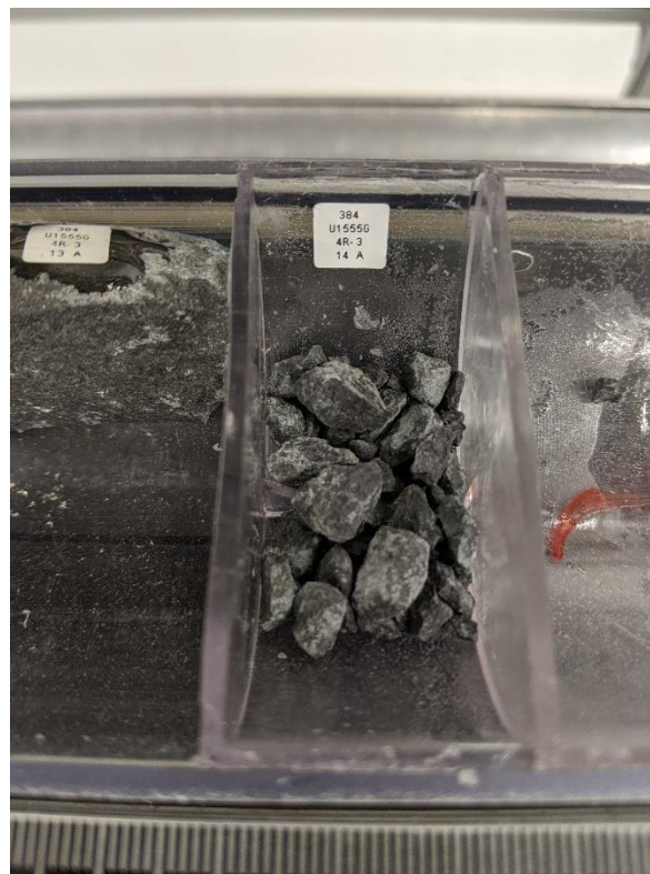
Figure 62. Examples of small hard rock samples that are labeled on the right side of the core liner because of their size
