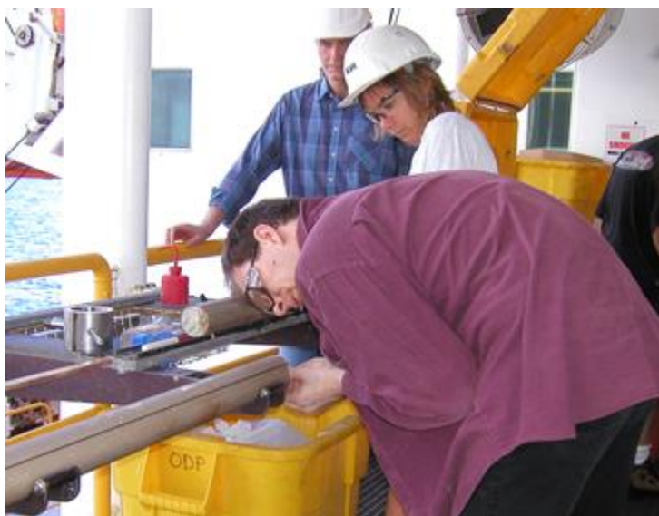
Figure 33. Example of Headspace gas sampling (HS)
