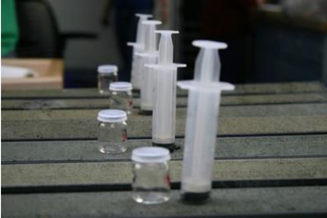
Figure 49. Syringes used to sample for moisture and density. Next to them are the properties beakers
