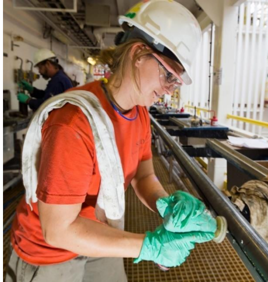
Figure 24. Drilling holes in liner
