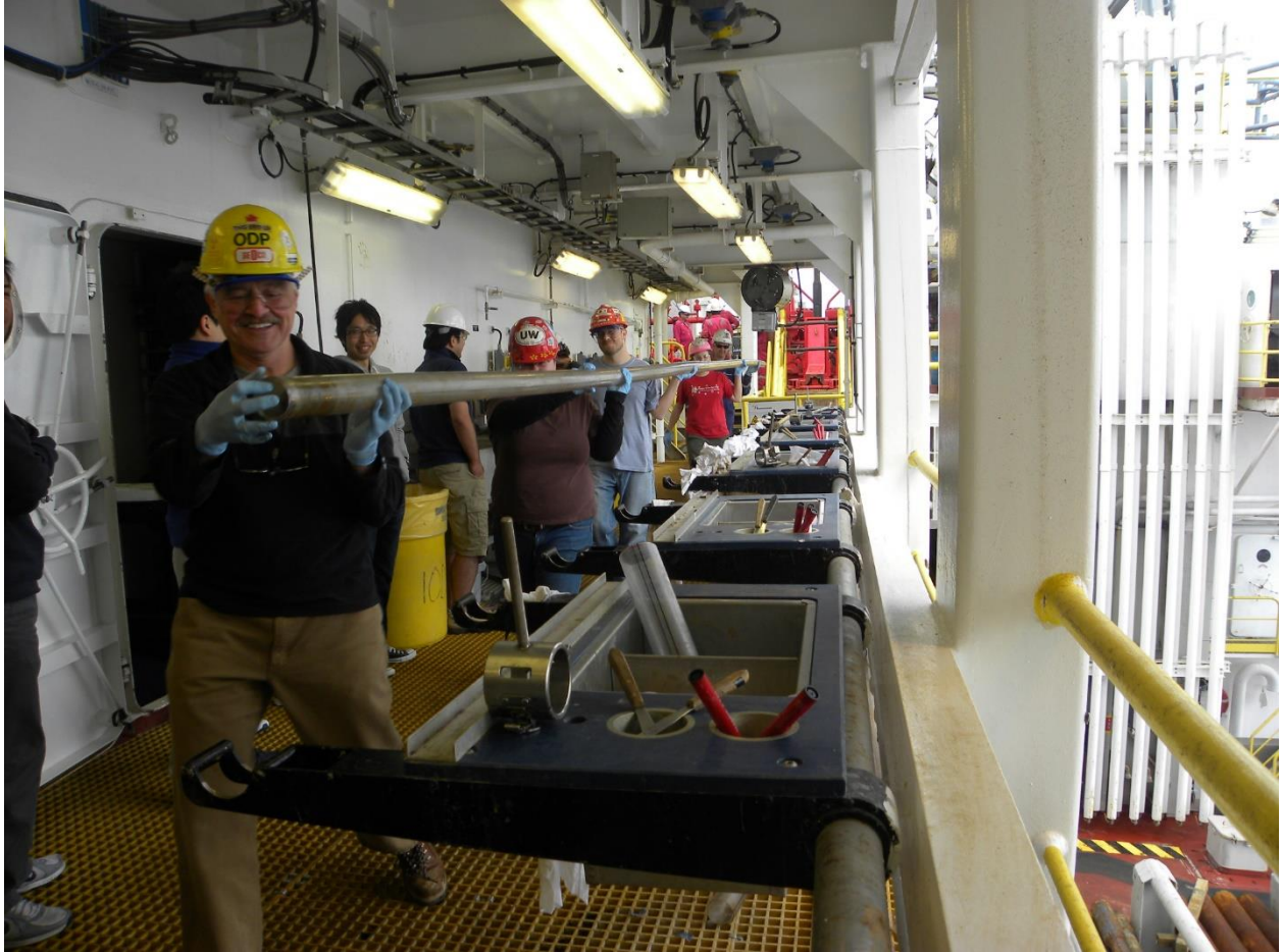
Figure 9. Crew holding the core in the Core Receiving Platform (“Catwalk)
