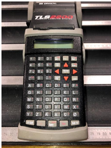
Figure 60. Brady Printer for hard rock labeling
