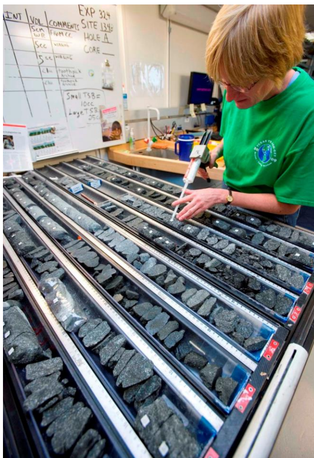
Figure 61. Gluing hard rock labels
