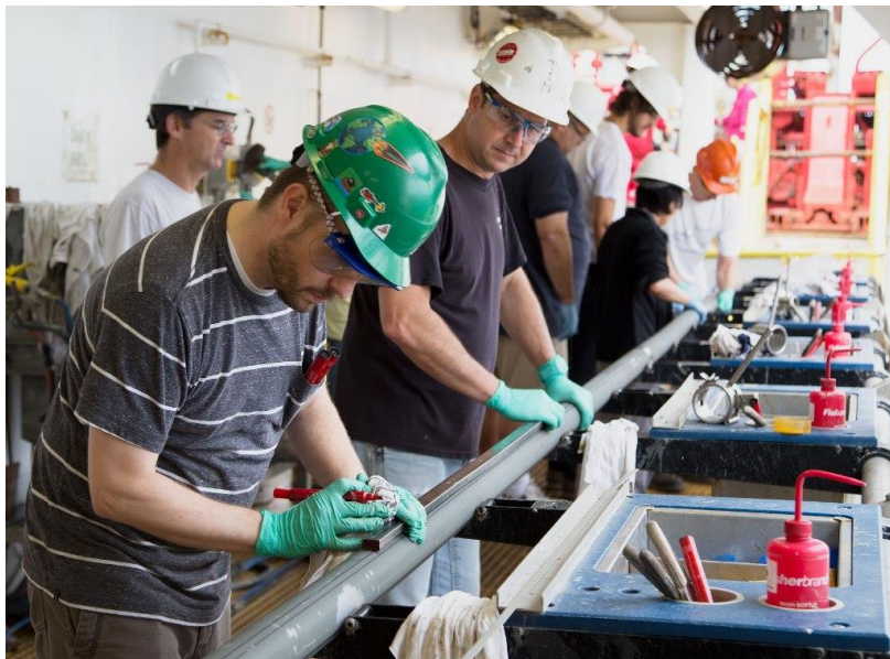
Figure 21. Marking liner at each 1.5 meters of core.
