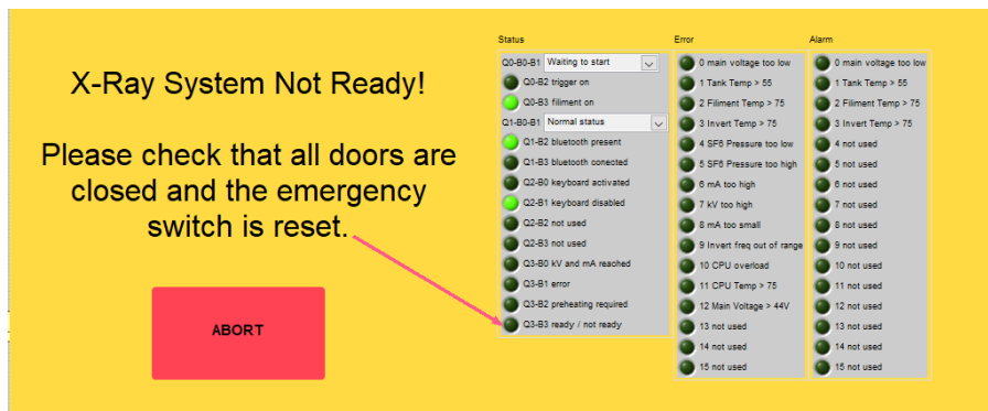
Figure 5. Warning message indicating that the source is not ready to ramp up.
