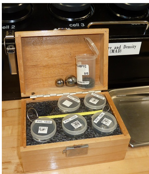
Figure 28. Six sets of steel balls are kept in this box along with the wire tool to extract them from the cells.
