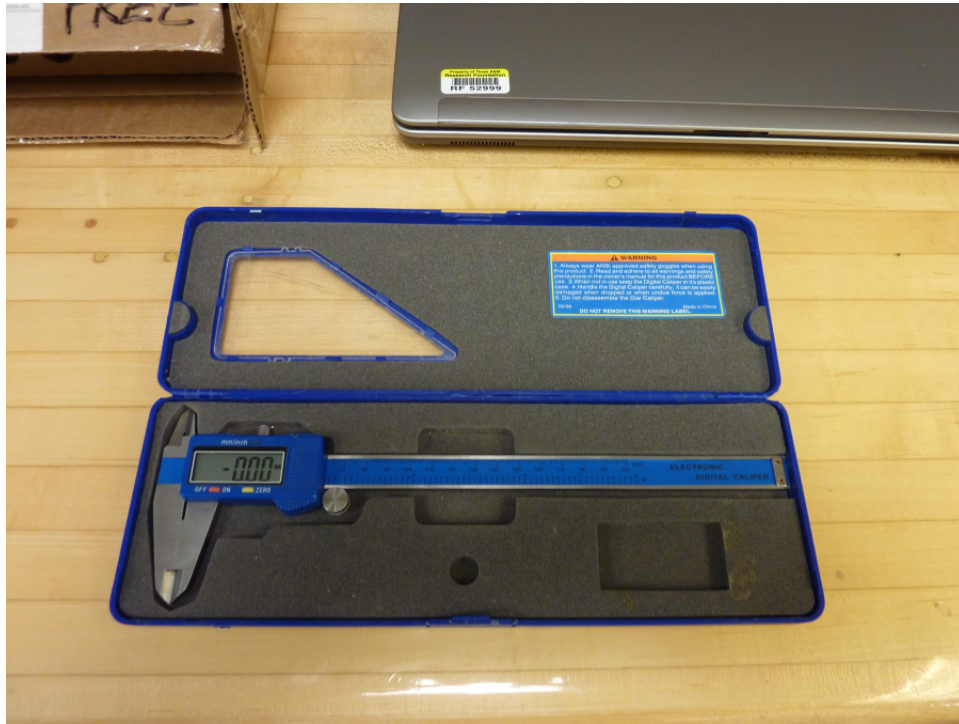
Figure 38. Precision Digital Caliper for measuring dimensions of certain samples.
