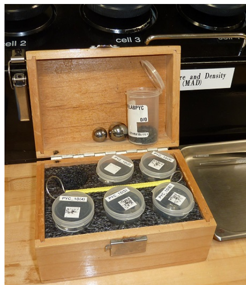
Figure 7. Six sets of steel balls are kept in this box along with the wire tool to extract them from the cells.
