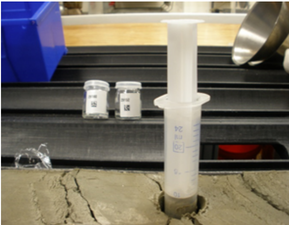
Figure 11a. Using cut-off syringe to get a 10ml sample. container, clean off debris around rim with a kim wipe.
