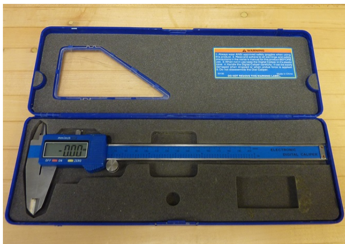
Figure 29. Digital caliper used for volume measurements.
