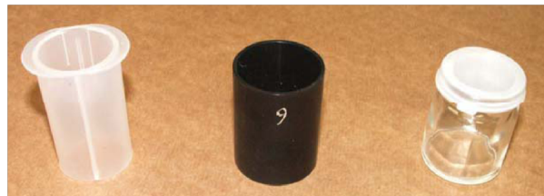
Figure 12. Sampling tool (left), aluminum cup, and Wheaton vial for MAD measurements.
