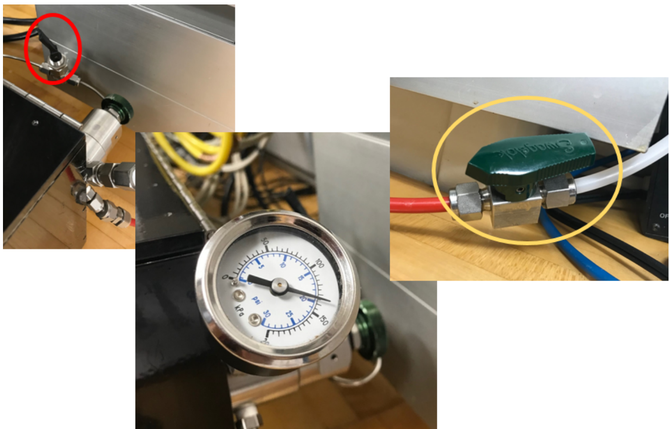
Figure 35. Regulator behind pycnometer (set to 19 psi). Both valves, before and after the regulator, should be open.
