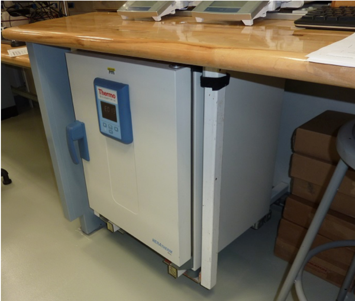
Figure 39. Thermo Scientific HERATHERM AP 60 L oven, mounted underneath the bench. Back-vented, the oven does not warm the benchtop and alter the results from the analytical balances.
