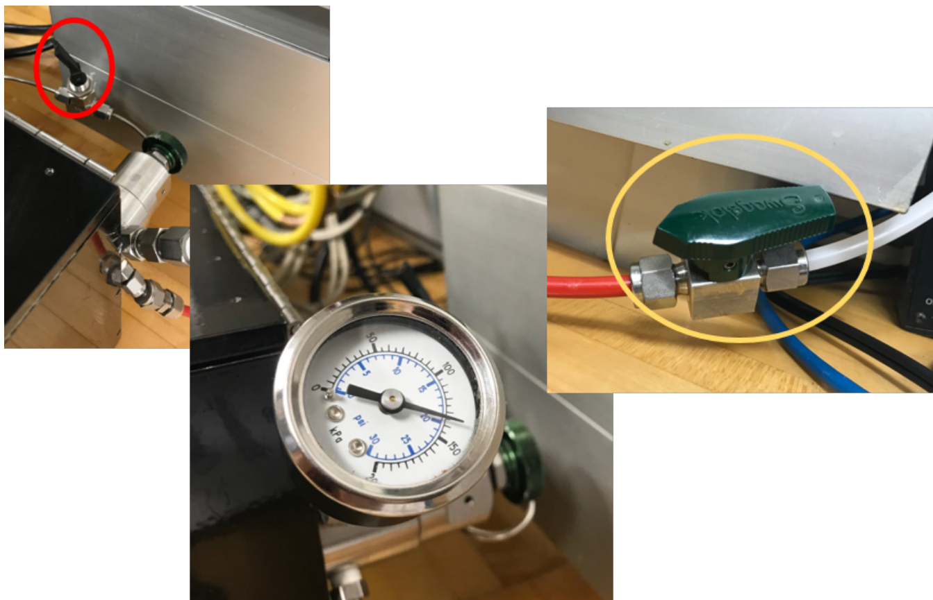
Figure 4. Regulator behind pycnometer (set to 19 psi). Both valves, before and after the regulator, should be open.
