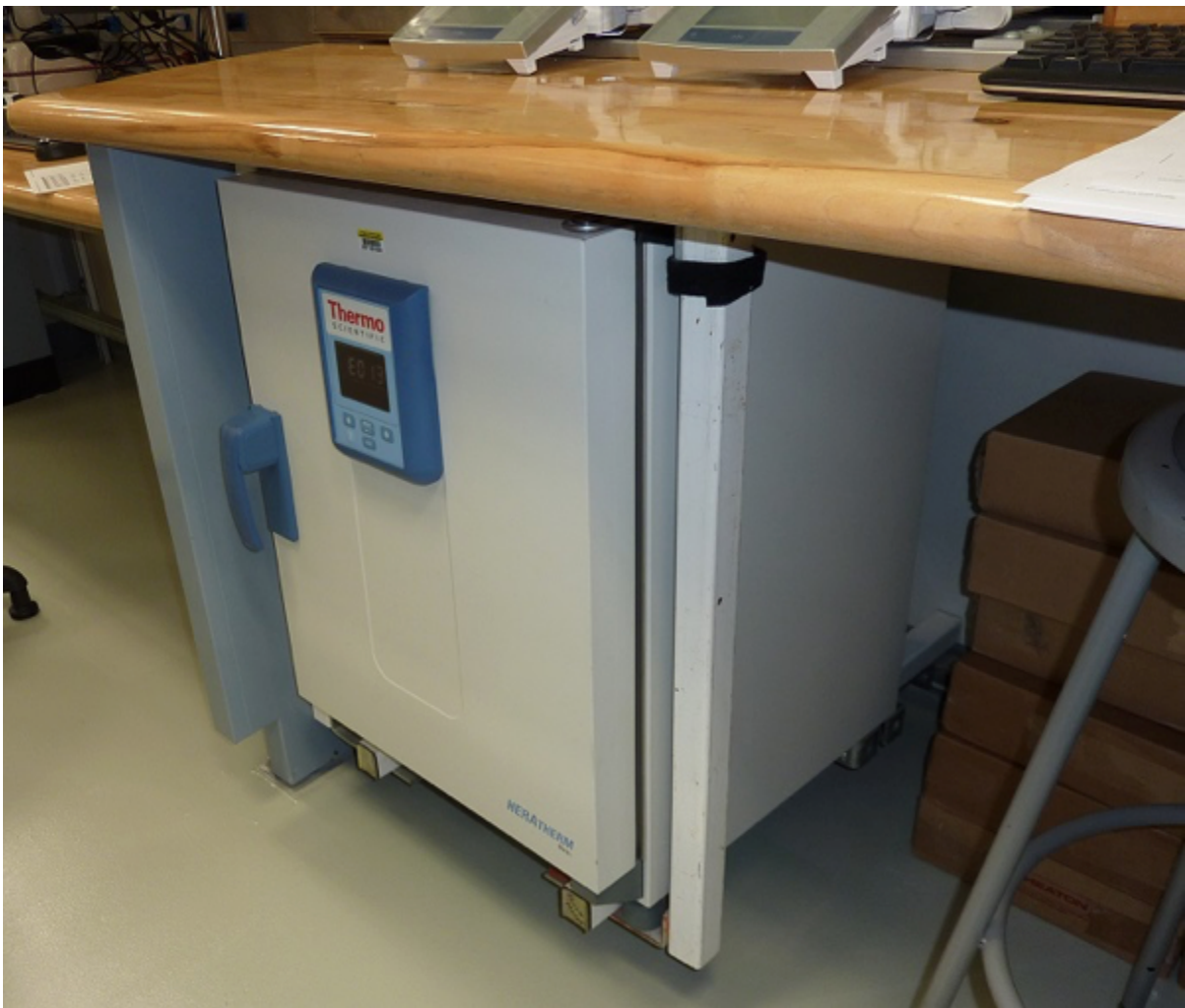
Figure 8. Thermo Scientific HERATHERM AP 60 L oven, mounted underneath the bench. Back-vented, the oven does not warm the benchtop and alter the results from the analytical balances.
