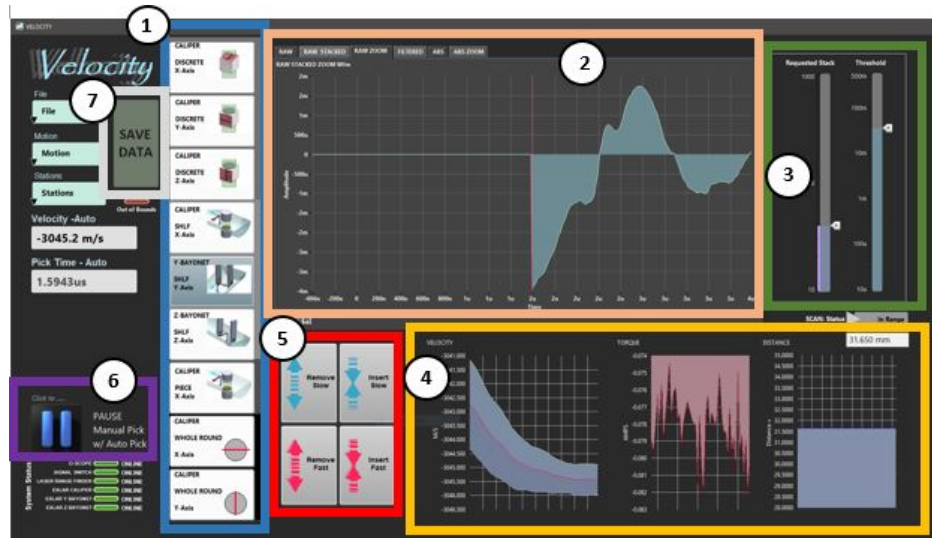
Figure 7: Main Velocity Window with annotated sections
