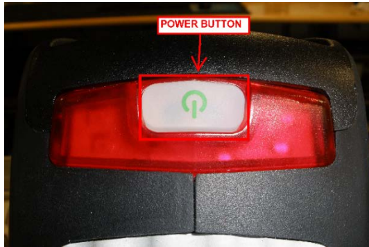
Figure 5. pXRF power button outlined in red. pXRF is off.
