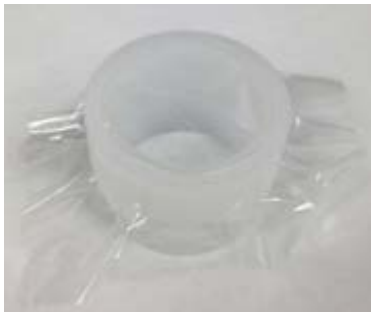
Figure 15. Ultralene® covering of one side of cup
