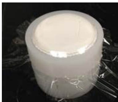
Figure 16. Properly filled XRF cup; note the slight bulge of the powder.
