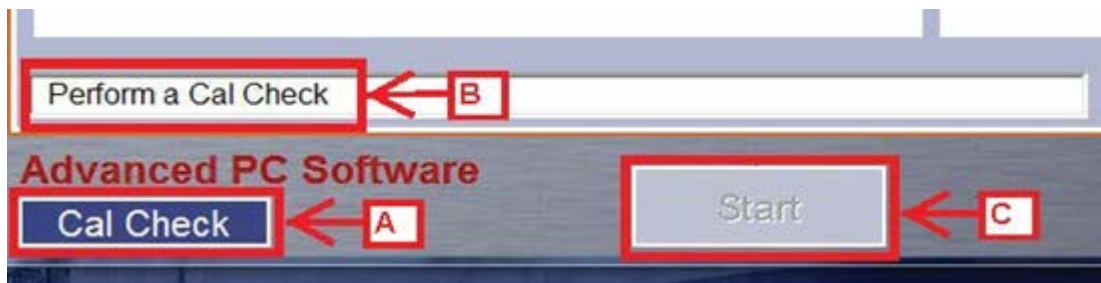
Figure 20. Performing a Calibration Check. A. CalCheck Button B. Indicator Bar C. Disabled 'Start' button
