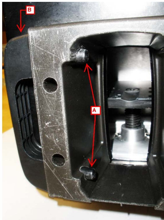
Figure 10. Bottom of Sample Chamber. A. Two pegs B. Release handle
